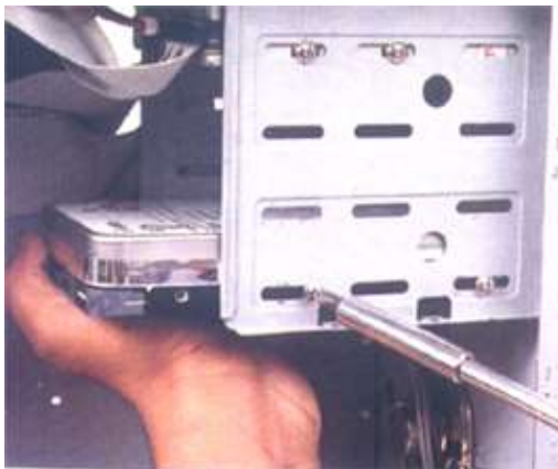
Fig 13.5 Fixing Harddisk in Cabinet
