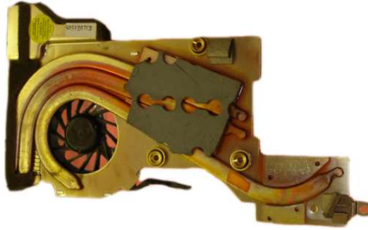
Fig 12.3 Heat Sink of Laptop
