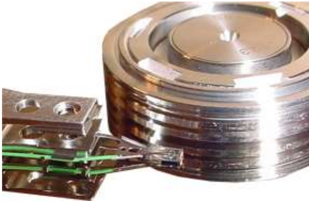
Fig 7.12 Inside view of ST35530A
