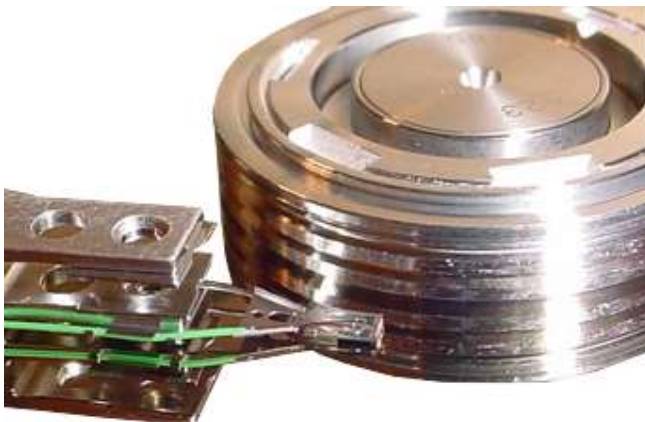
Fig 2.9 Multi disk single head system in a Hard disk
